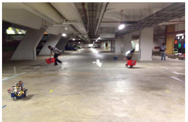
Fig. 3. A picture taken during the experiment. Two pedestrians are crossing the overlapped sensor FOVs at the same time.
