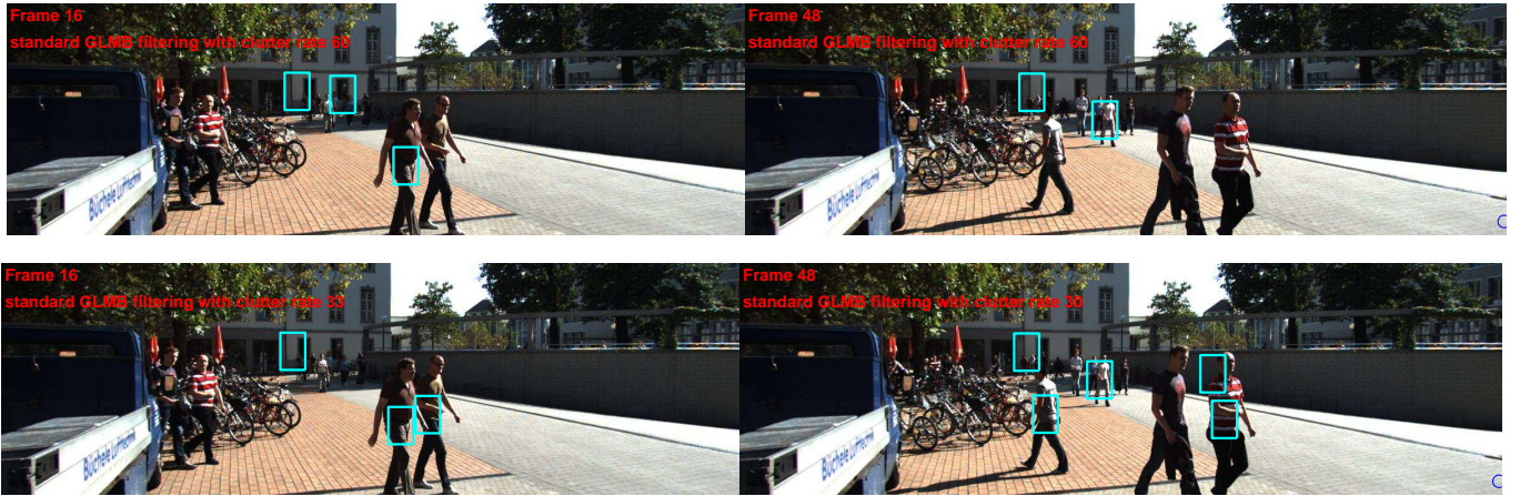
Fig. 1: Frames 16, 48 of the image sequence from [5] and object detections obtained using the detector in [40]. The number of objects varies with time due to objects coming in and out of the scene. Object estimates (marked by blue boxes) using the standard GLMB filter for guessed clutter rate of 60 (left column) and ‘true’ clutter rate (right column). Tracking using ‘true’ clutter rate accurately estimated several objects that were missed in the frames on the left.
