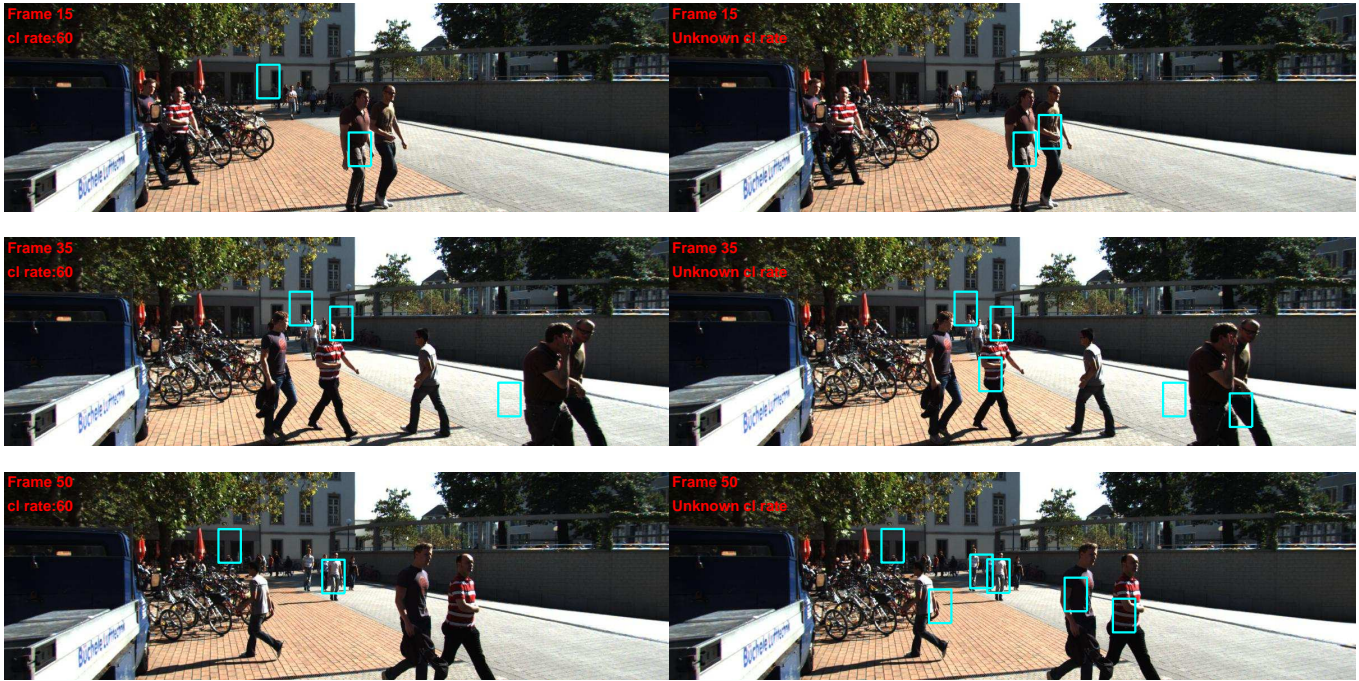
Fig. 9: Tracking results for frames 15, 35, 50 with guessed clutter rate 60 (left) and the proposed filter (right) for dataset 2.
