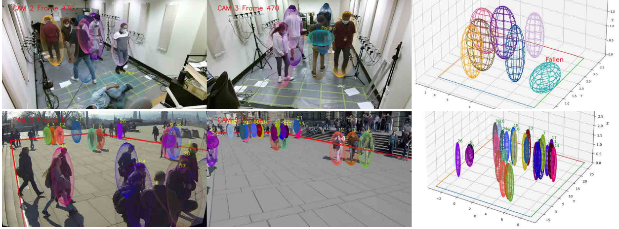
Figure 4: 3D ellipsoid estimates from the proposed MV-GLMB-AB filter using CStrack detection inputs. Top row: CMC5 dataset at frame 470 for cameras 2 and 3. Bottom row: WT dataset at frame 25 for cameras 2 and 5 (only objects inside the red boundary are considered). The first two columns show the projected 3D estimates on the respective camera planes, and the last column shows the 3D estimates. Each color corresponds to a unique object ID. Videos are also provided in the supplementary materials.
